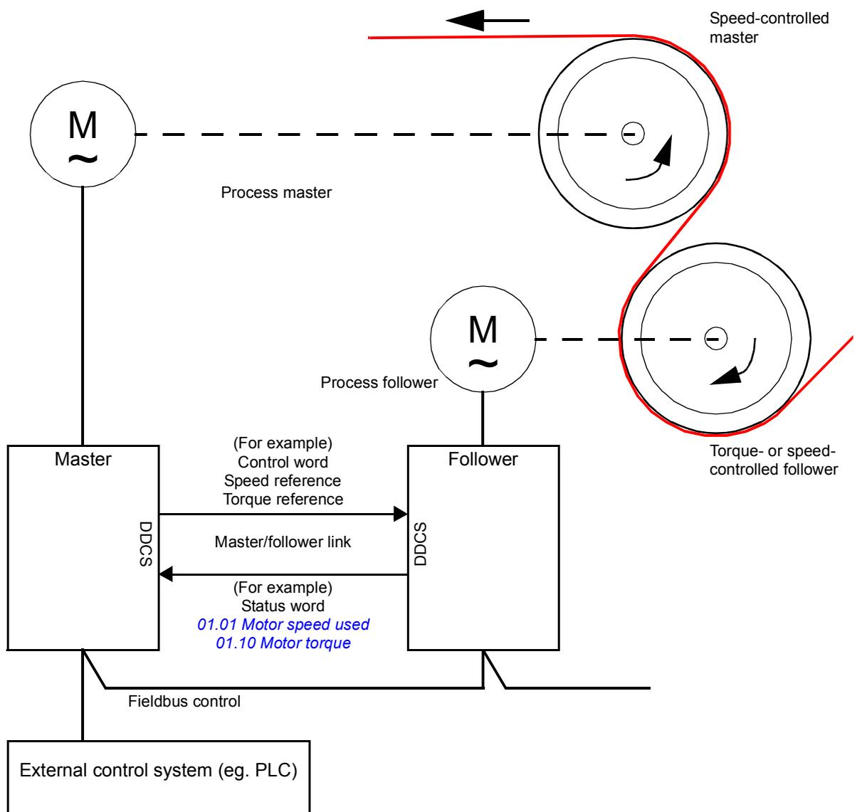
The master drive is typically speed-controlled and the other drives follow its torque or speed reference. In general, a follower should be
