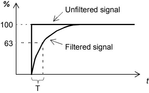
$O = I \times (1 - e^{-t/T})$ <p>I = filter input (step)<br/> O = filter output<br/> t = time<br/> T = filter time constant</p> | 0.100 s    |
