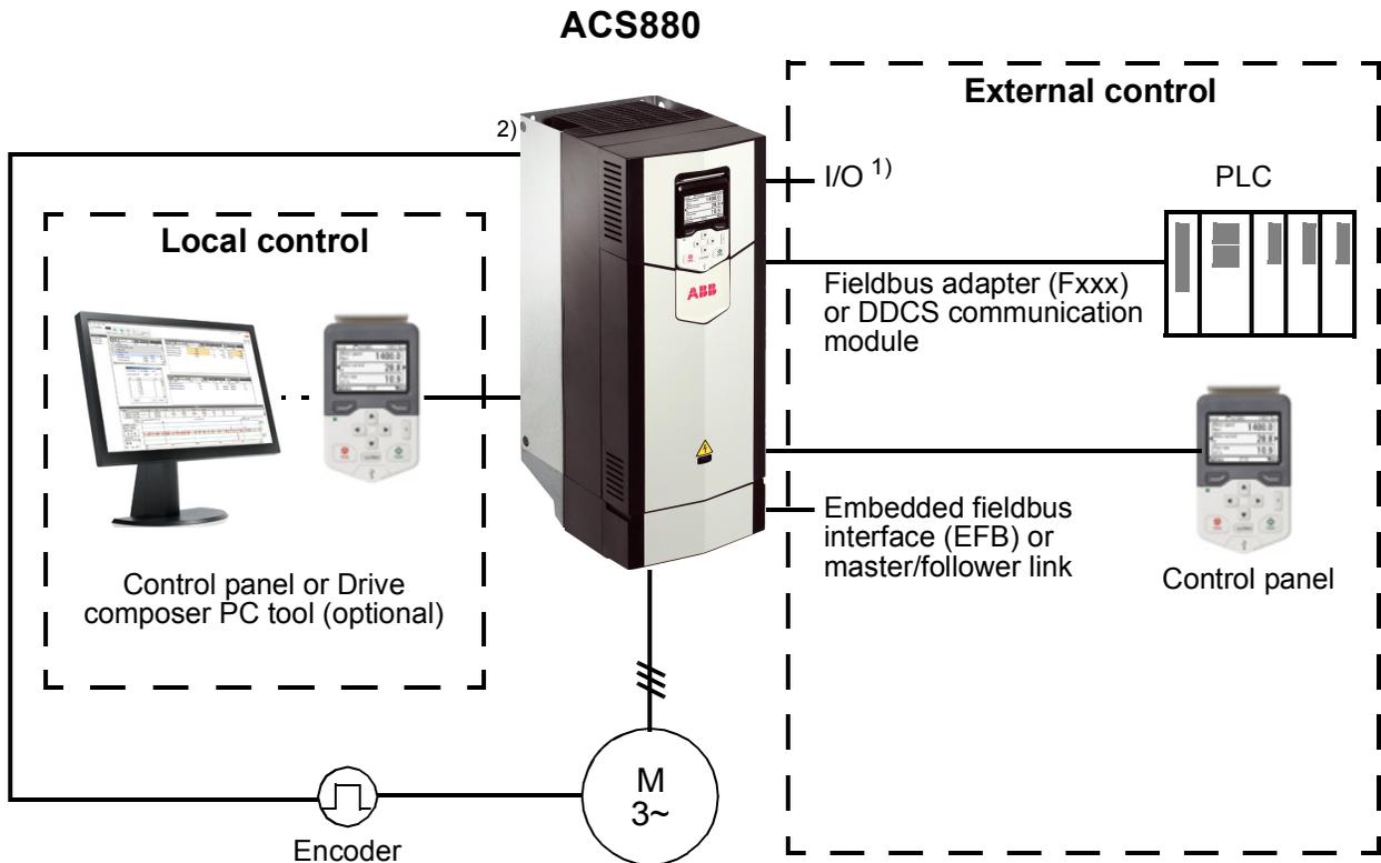
1) Extra inputs/outputs can be added by installing optional I/O extension modules (FIO-xx) in drive slots.
