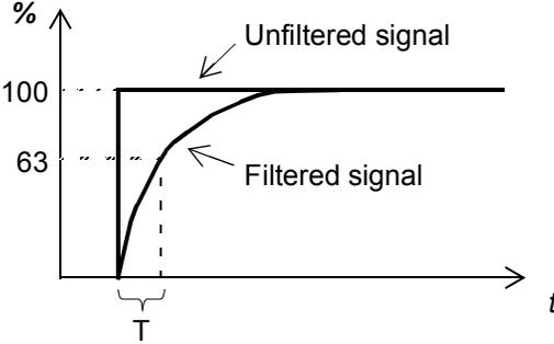
$O = I \times (1 - e^{-t/T})$ <p>I = filter input (step)<br/>O = filter output<br/>t = time<br/>T = filter time constant</p> <b>Note:</b> The signal is also filtered due to the signal interface hardware. See parameter 14.46 AI2 filter gain.                                                             | 0.100 s    |
