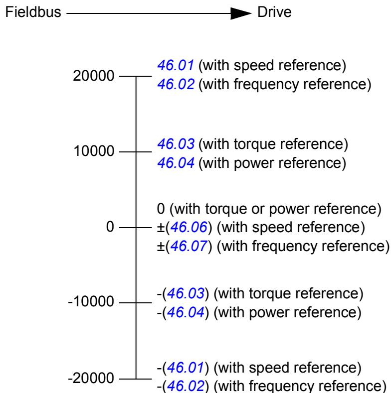
The scaled references are shown by parameters [03.09 EFB reference 1](#) and [03.10 EFB reference 2](#).
