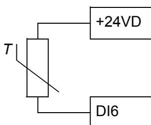
The resistance of the PTC sensor increases when its temperature rises. The increasing resistance of the sensor decreases the voltage at the input, and eventually its state switches from 1 to 0, indicating overtemperature.
