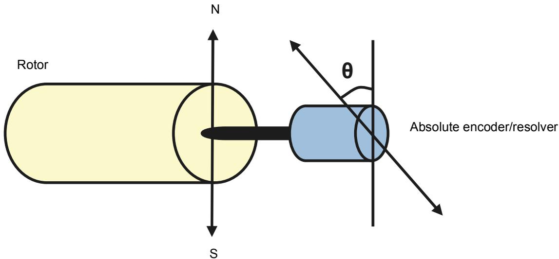
The autophasing routine is performed with permanent magnet synchronous motors and synchronous reluctance motors in the following cases:
