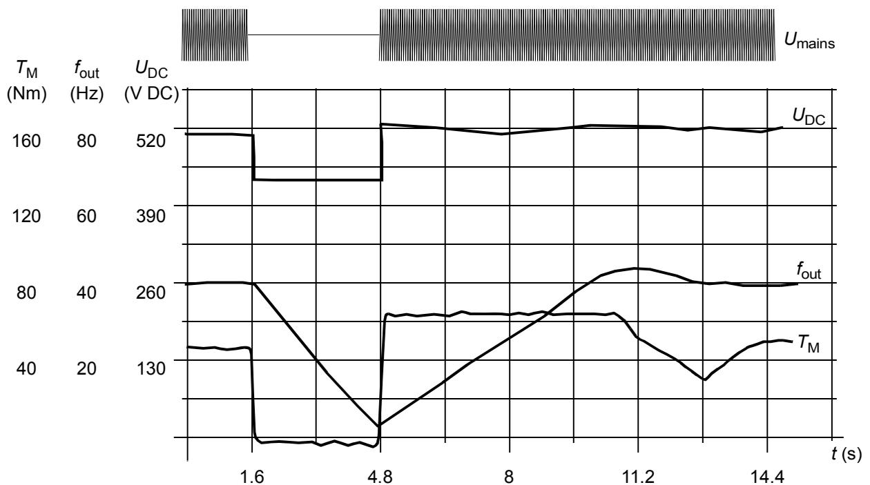
$U_{DC}$  = intermediate circuit voltage of the drive,  $f_{out}$  = output frequency of the drive,  $T_M$  = motor torque
