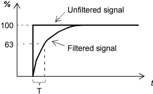
$O = I \times (1 - e^{-t/T})$ <p>I = filter input (step)<br/> O = filter output<br/> t = time<br/> T = filter time constant</p> <p><b>Note:</b> The signal is also filtered due to the signal interface hardware. See parameter 14.61 AI3 filter gain.</p> | 0.100 s          |
