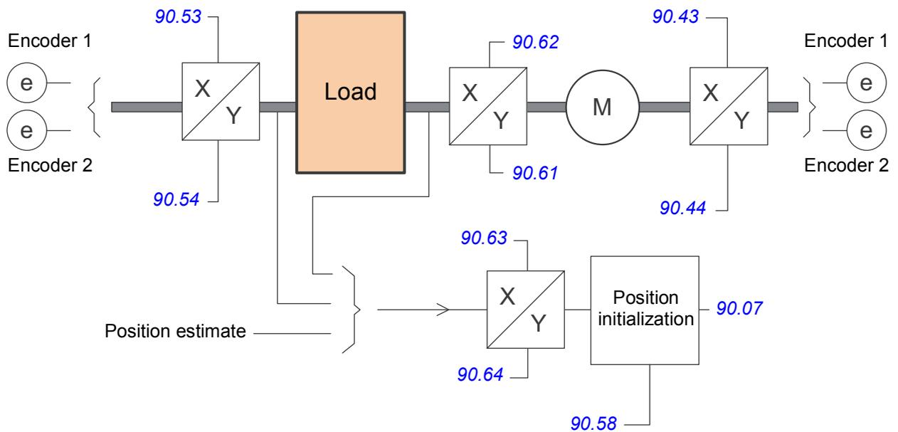
The source of the measurement is selected by [90.51 Load feedback selection](#). Any gear ratio between the encoder and load is defined by [90.53 Load gear numerator](#) and [90.54 Load gear denominator](#). In case the internal position estimate is chosen as the source, the gear between the motor and load must be defined in [90.61 Gear numerator](#) and [90.62 Gear denominator](#).
